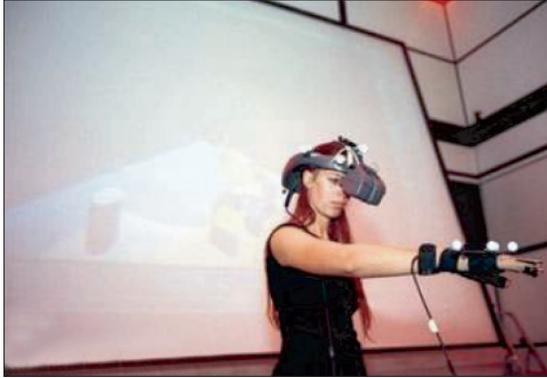
**Fig. 1.** Head-mounted display and haptic glove
