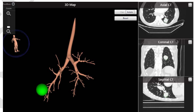
Figure 2. SuperDimension Navigation System 3D Map – Determining the position of the pathological mass in relation to the airways.
